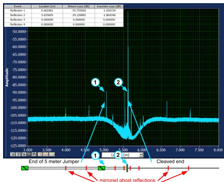
Figure 12 A close-up of Rayleigh Scatter versus position of a jumper with a cleaved end
