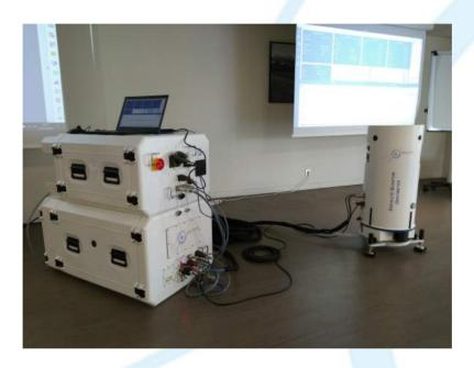
Based on the same technology as the AQG, the Field AQG belongs to the family of automated and turn-key absolute gravity sensor based on laser-cooled atoms. This ruggedized and temperature -controlled version meets the objective to provide the excellent measurement performances of Muquans quantum gravimeter even when operating outdoor.
