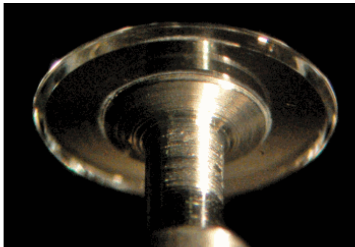
A crystalline WGM microresonator made of \text{CaF}_2 has an unloaded Q factor of 2 \times 10^9 . Its extremely high Q results in significant surface Rayleigh backscattering (the lower the losses
